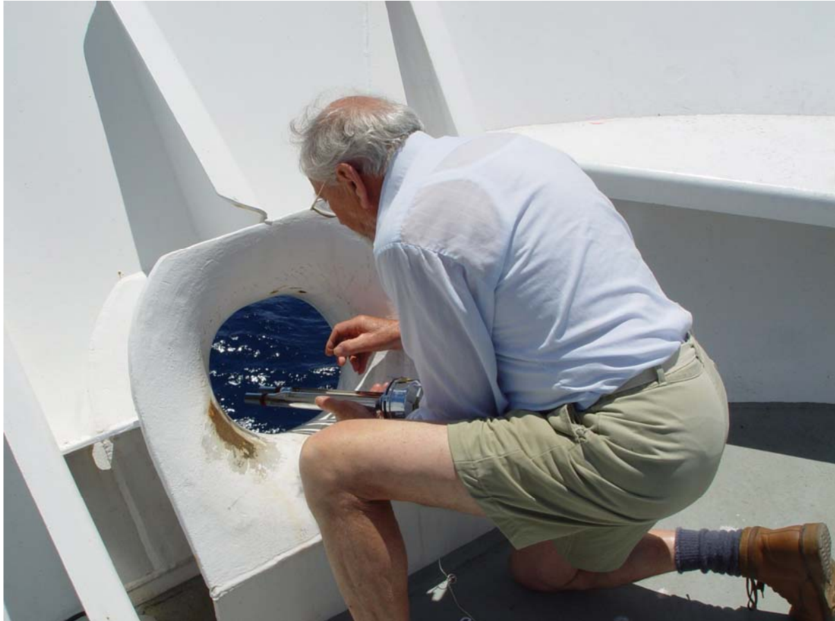
Figure 3.1. Measuring wet and dry bulb temperatures with an Assman ventilated psychrometer. The use of the forward chock as a sampling location ensures good exposure and some shielding from the sun.
