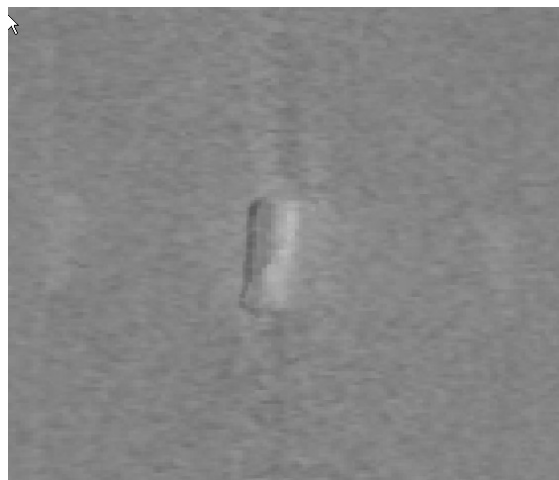
Figure 3. Screen grab showing EM 302 seabed backscatter data collected over the wreck surveyed on 9/18/11. Image created in IVS FMGT.
