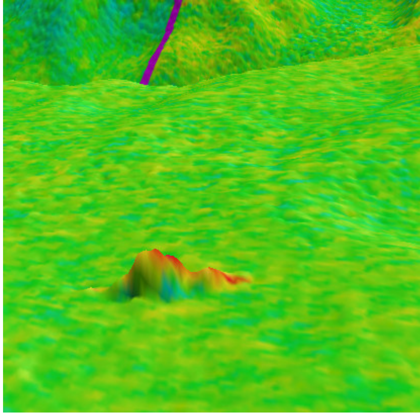
Figure 17. Oblique view looking southwest, showing EM 302 multibeam bottom backscatter data of a possible wreck in Block Canyon. Mosaic cell size 5 meters. Red indicates stronger acoustic return signal.
