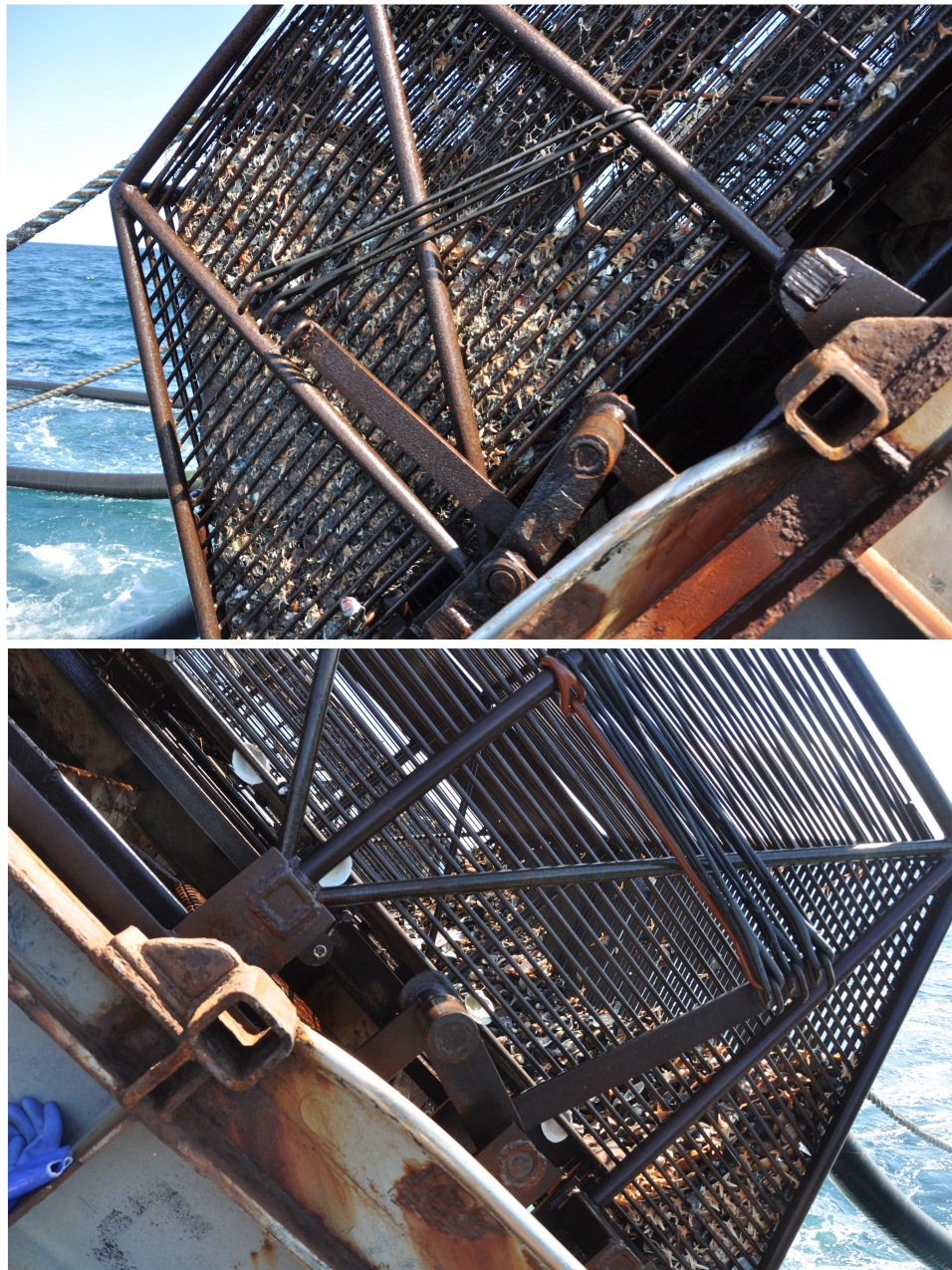
Figure 5. The catch in the lined dredge (above) and the Dameron-Kubiak dredge (below) when both were towed for 2 min over the same ground.
