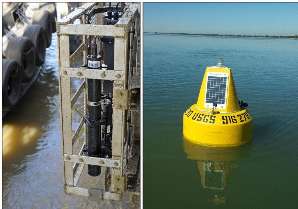
Figure 2-2. (L) shows a Sea-Bird Scientific SUNA V2 (Submersible Ultraviolet Nitrate Analyzer) mounted on a fixed structure on the Mississippi River at Baton Rouge, where the instrument cage is lowered and raised. (R) shows a NexSens buoy supporting a Sea-Bird Scientific SUNA nitrate sensor and WET Labs Cycle Phosphate sensor (in addition to a YSI EXO multi-parameter sonde measuring algal pigments, turbidity, and dissolved organic matter). (Photos courtesy of Brian Pellerin/USGS)
