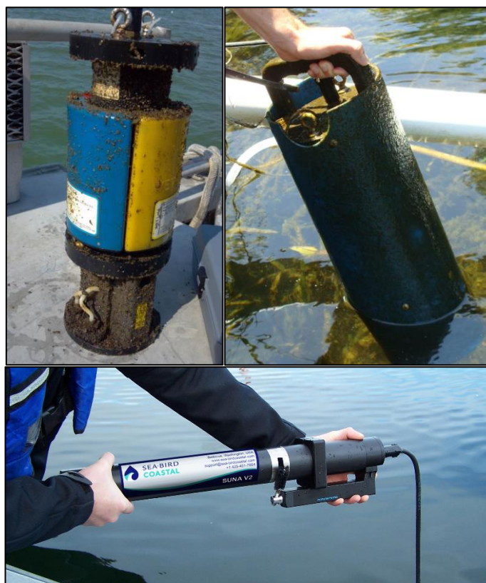
Figure 2-7. These Sea-Bird Scientific Cycle PO4 phosphate sensors have accumulated an external bio-fouling coating during deployment (top). A Sea-Bird Scientific SUNA nitrate sensor uses a rotating, motorized brush to keep the optical lenses free of bio-fouling. (Photos courtesy of Corey Koch/WET Labs)
