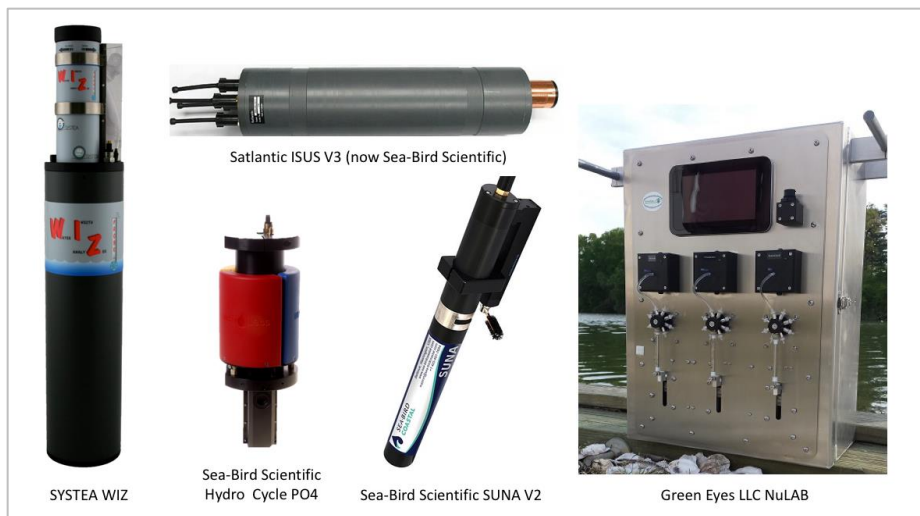
Figure 2-6. Commonly used DN sensors. (Photos courtesy of Corey Koch/WET Labs, Pompeo Moscetta/SYSTEA, and Vince Kelly/Green Eyes LLC)
