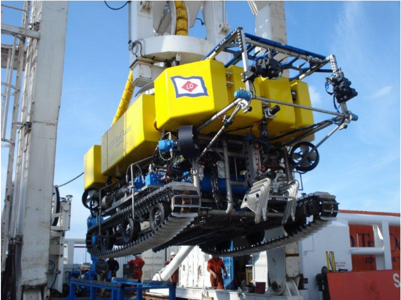
Figure 5. A 400 series ROVJET, an ROV proposed for use in Quintillion's subsea fiber optic cable network project, Bering, Chukchi, and Beaufort Seas, Alaska.
