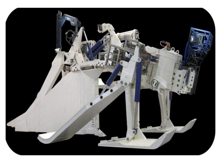
Figure 4. An SMD HD3 plough, a heavy duty subsea plow proposed for use in Quintillion's subsea fiber optic cable network project, Bering, Chukchi, and Beaufort Seas, Alaska.
