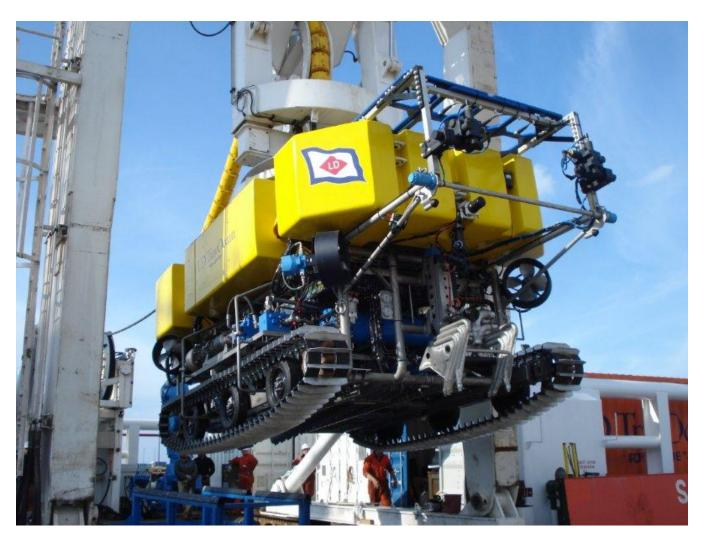
Figure 5. A 400 series ROVJET, an ROV proposed for use in Quintillion's subsea fiber optic cable network project, Bering, Chukchi, and Beaufort Seas, Alaska.
