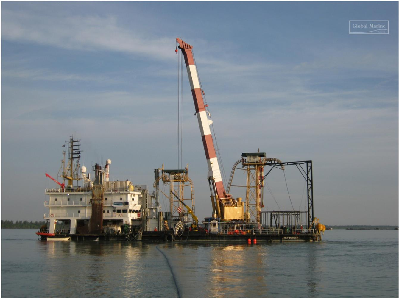
**Figure 3. The *CB Networker*, a cable-laying barge proposed for use in Quintillion's subsea fiber optic cable network project, Bering, Chukchi, and Beaufort Seas, Alaska.**
