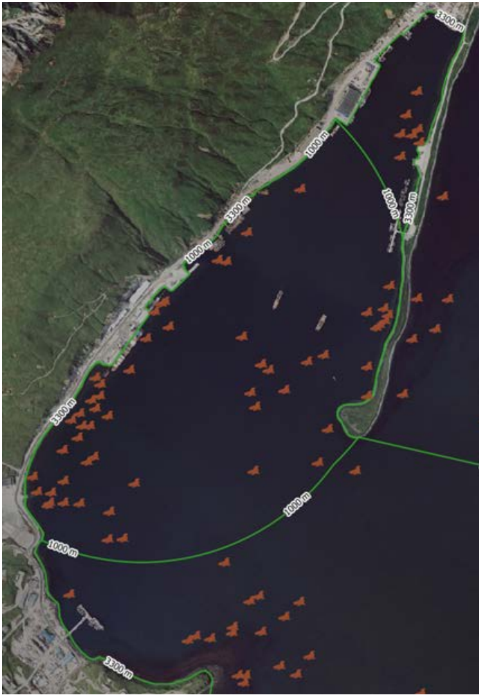
Figure 11. Steller sea lions observed in the action area from August-September, 2015 to June-July, 2016 (PND 2016). Also shows modeled radius of 120-dB isopleth (3,300 m) for vibratory pile-driving and removal and modeled radius of 160-dB isopleth (1,000 meters) for impact pile driving for the UMC Dock Positions III and IV replacement project, Dutch Harbor, Unalaska, Alaska.
