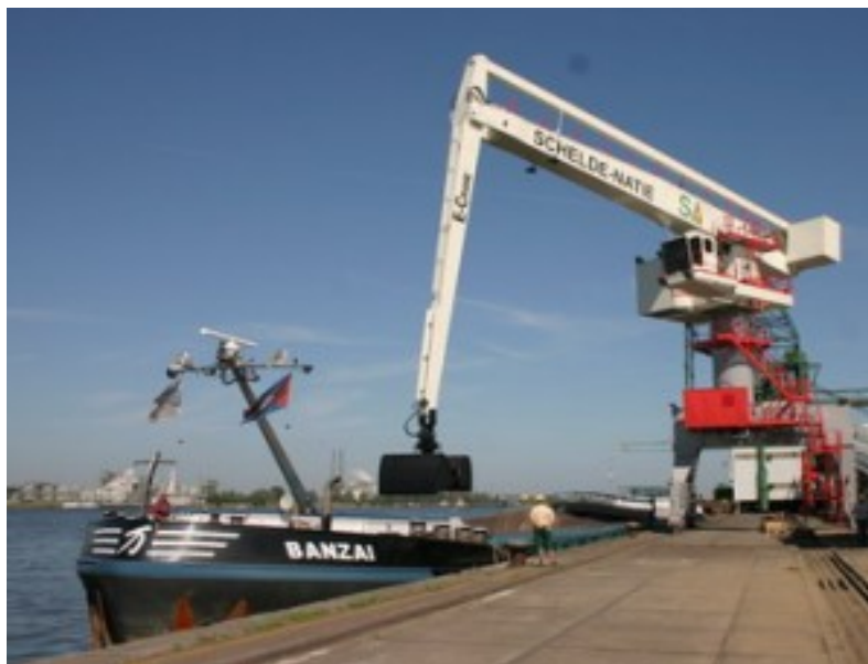
Figure 3. Example image of a crane used to load and unload vessels, which can move across dock area on rails.
