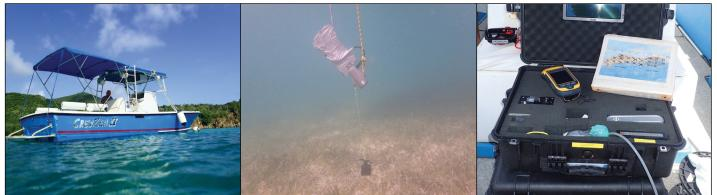
Figure 2.8. Equipment used to collect GV and AA data in the field: (left) small boat used to access sites, (middle) Seaviewer HD video drop camera setup, and (right) topside system, including a GPS, monitor and video recording.
