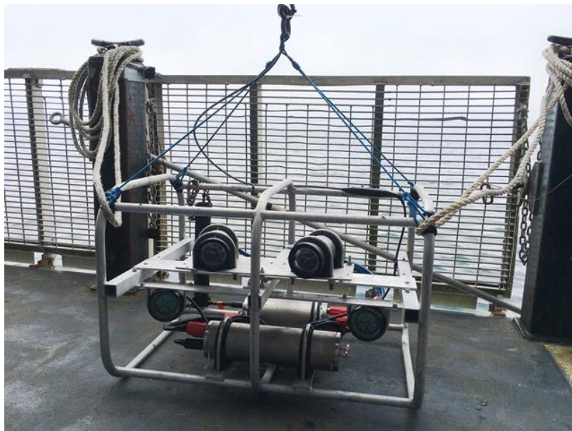
App. 6, Fig 4. – Lowered stereo camera for krill. Winch and deployment are same as in Appendix 3.
