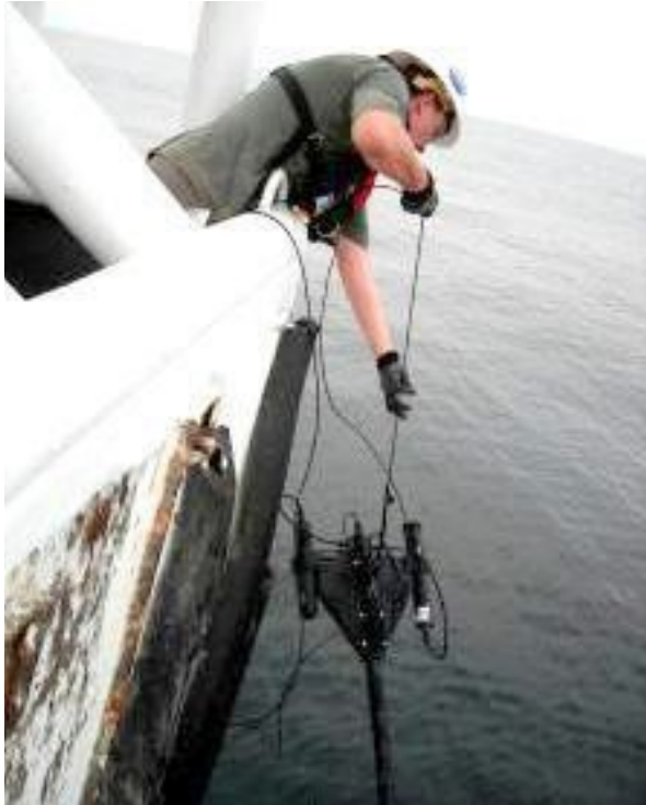
Figure 6. Submersible radiometer being hand-deployed .
