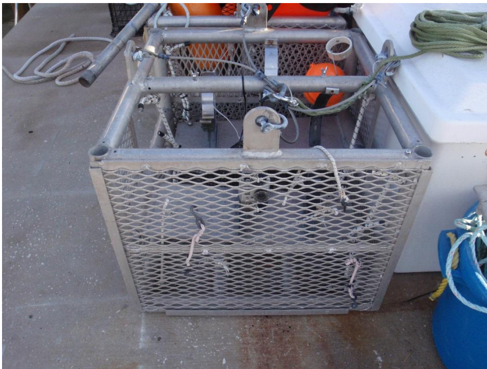
Figure 4. Stereo camera pod. Two cameras are placed inside, each facing 180° to the other. There are also GoPro cameras positioned on the adjacent sides to record surrounding habitat; the four cameras together provide a 360° view.
