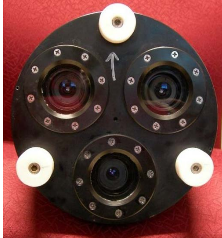
Figure 3. Forward view of camera system. Upper cameras are pair of fixed-distance stereo still cameras while single bottom camera is digital video camera. Files are recorded for both: 1) folder of left and right bitmap images (~1440 per 30 min. deployment) and 2) folder of .mp4 videos (~3-4 per 30min. deployment).
