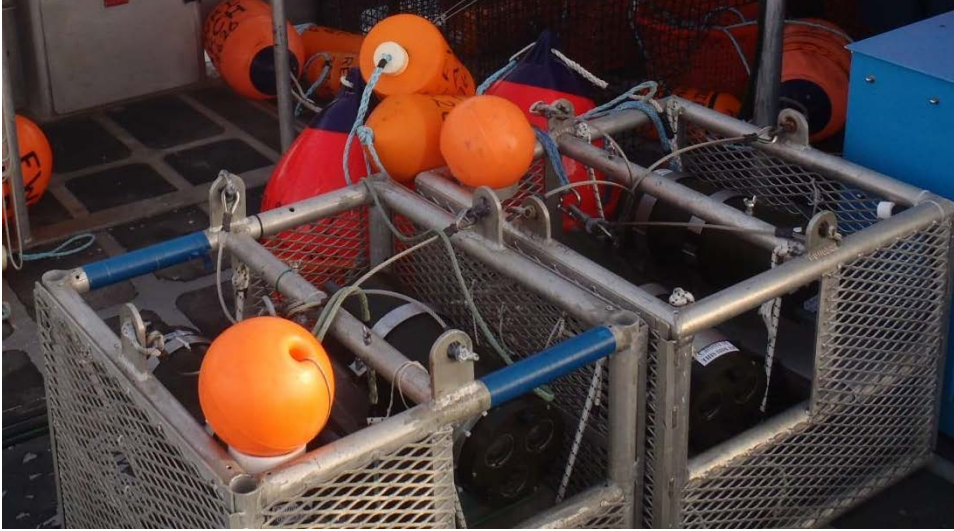
Figure 5. Stereo camera pods (2) with cameras mounted inside. Camera arrays are deployed with 12-strand AmSteel line to a surface buoy. They are retrieved using ships' hydraulics.
