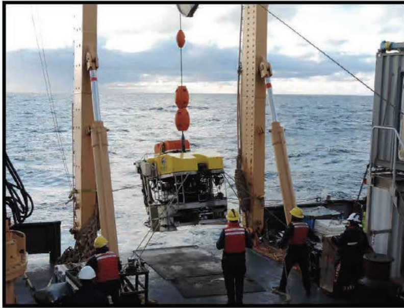
Example of Tag Lines used during launch and recovery
