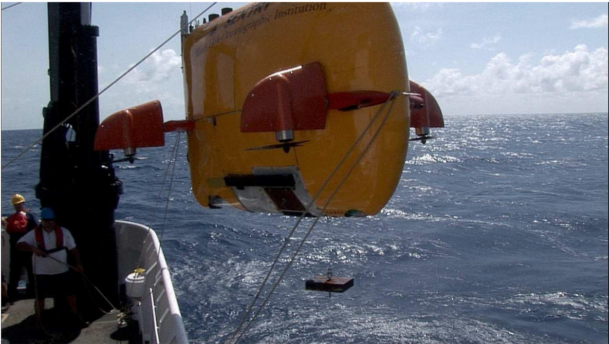
Figure 9 - As Sentry moves over the rail, the forward tagline is slacked and slipped.
