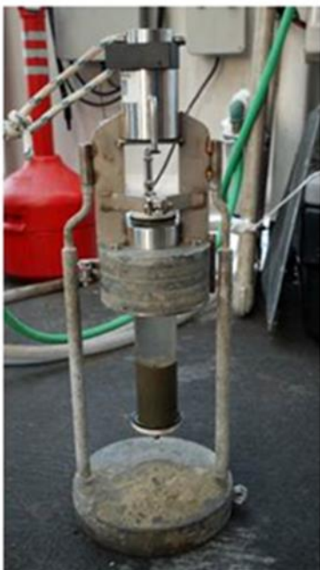
Figure 3. NIOZ moncore will be suspended under the CTD rosette by a 10 m line. The moncore weighs about 33 lbs.
