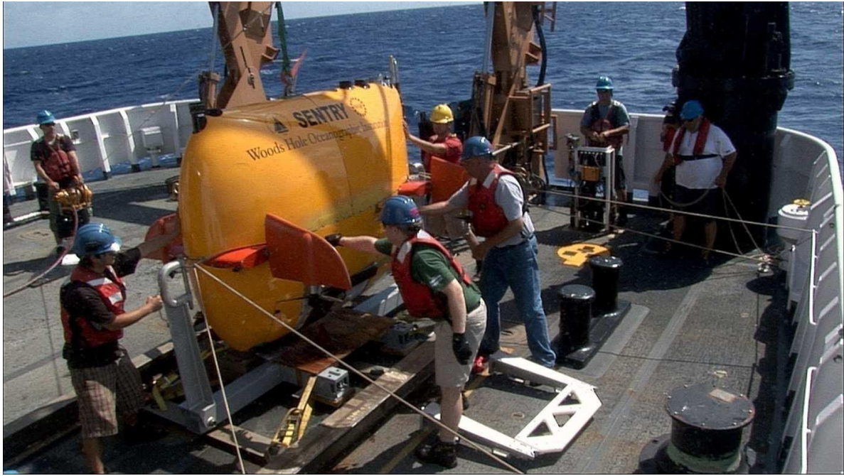
Figure 6 - The outboard side of the cradle is removed and the pipes through the center of the vehicle are removed.
