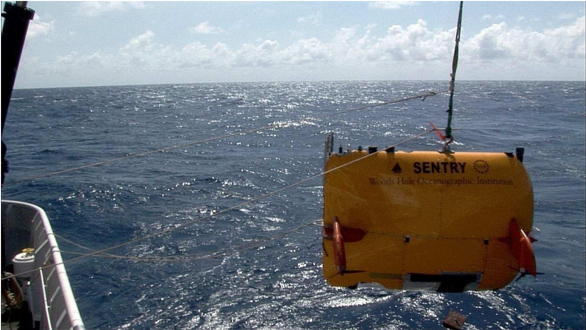
Figure 9 - As Sentry moves over the rail, the forward tagline is slacked and slipped.
