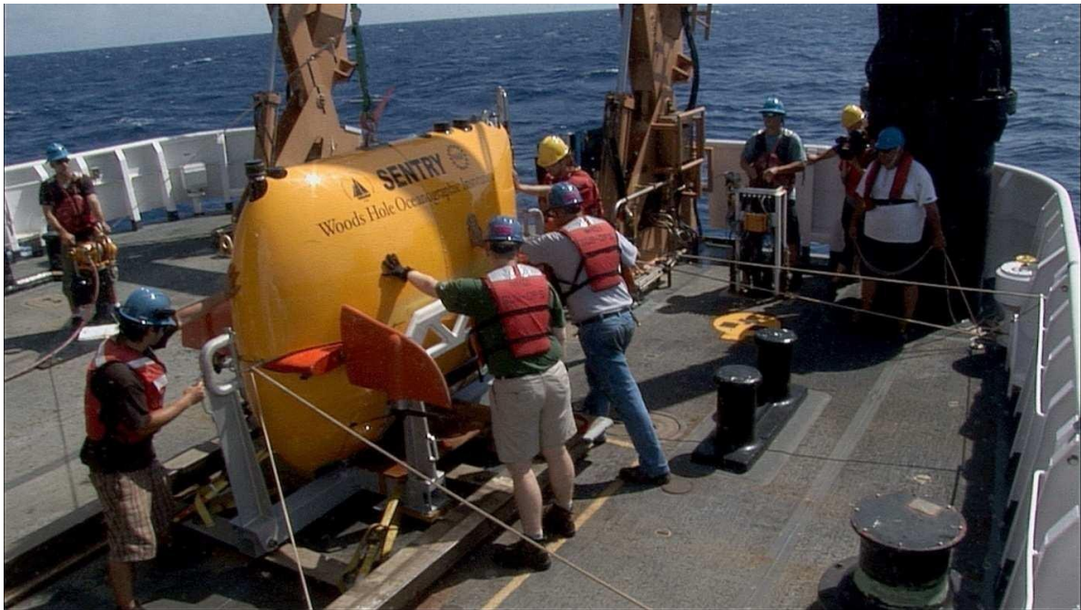
Figure 5 - Sentry is in the cradle and lifted approximately 1-2 inches
