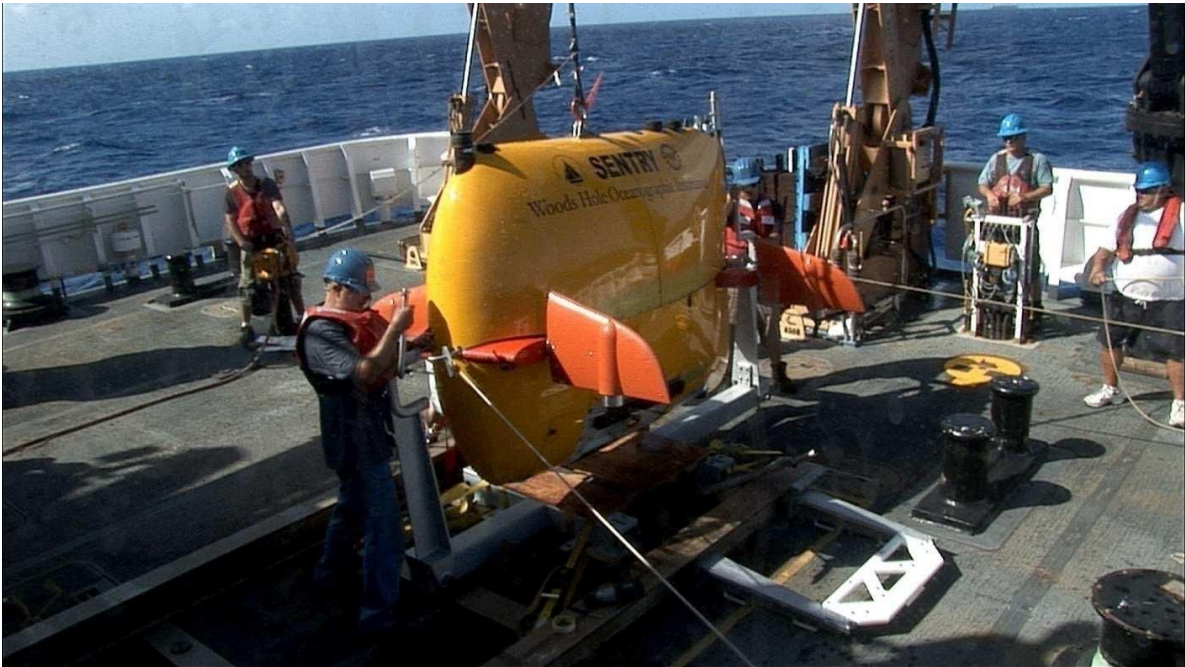
Figure 13 - The vehicle is slewed back into the cradle and the fore and aft catches are secured first. The side is reattached and the poles reinserted before the vehicle is set into the cradle.
