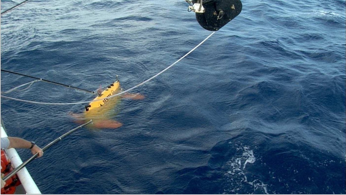
Figure 11 - As the vehicle drives towards the stationary vessel, the lift line for the crane is attached using a carbon fiber pole. The vehicle immediately drives full reverse and the pole is potentially used to fend the vehicle while the lift line is tensioned.
