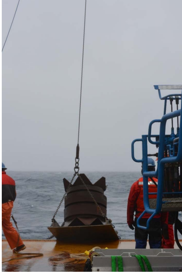
(Flanking mooring anchor being tipped over the stern)
