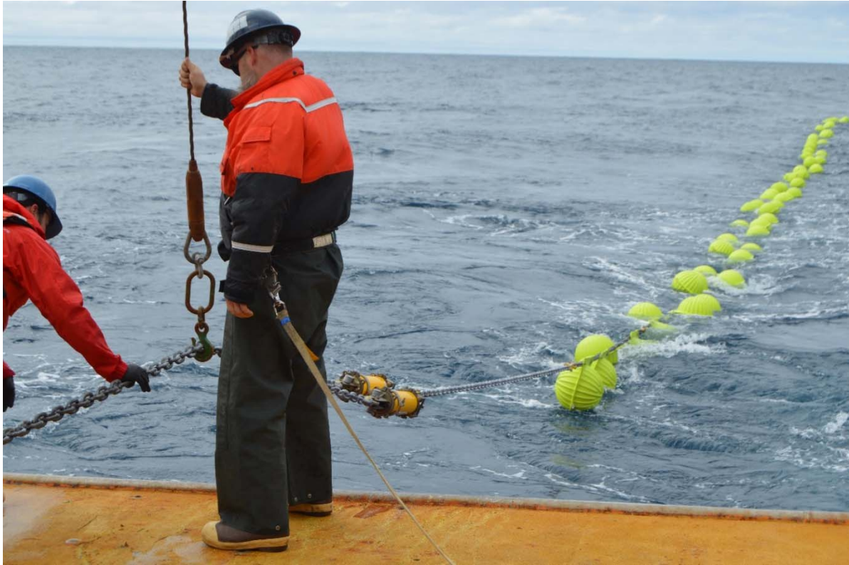
(Backup Recovery Flotation and Releases)
