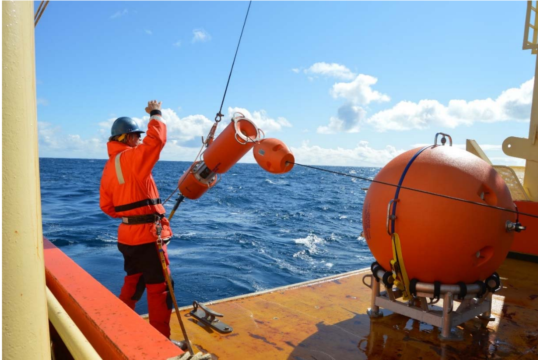
(Deployment of Upper Release Module)
