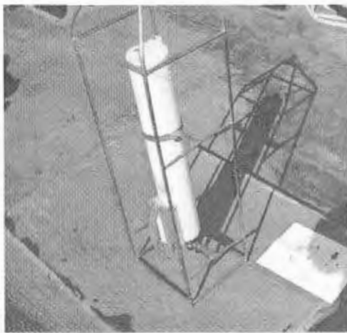
Figure 4: Conductivity, temperature and depth instrument inside cage
