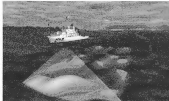
Figure 1: Multibeam swath sonifying the seafloor
