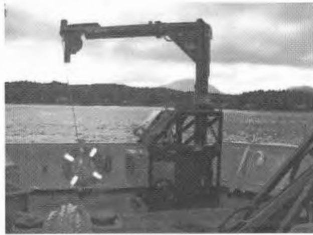
Figure 5: Moving vessel profiler mounted on fantail
