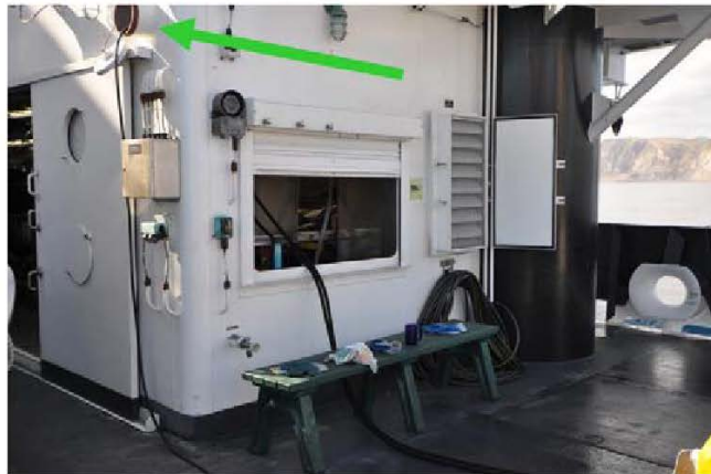
Figure 1a. Photo from fantail of aft entrances to wet lab. The HPU hoses are currently run out of the roll-up door. The green arrow points to the bulkhead opening which would be the preferred route for the HPU hoses.
