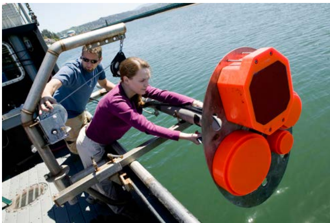
Figure B1: Example of an over-the-side-pole for small-boat acoustics operations.
