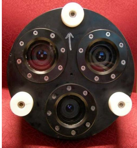
Figure 5. Forward view of camera system. Upper cameras are pair of fixed-distance stereo still cameras while single bottom camera is digital video camera. Files are recorded for both: 1) folder of left and right bitmap images (~1440 per 30 min. deployment) and 2) folder of .mp4 videos (~3-4 per 30min. deployment).
