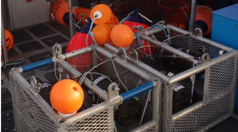
Figure 7. Stereo camera pods (2) with cameras mounted inside. Camera arrays are deployed with 12-strand AmSteel line to a surface buoy. They are retrieved using ships' hydraulics.
