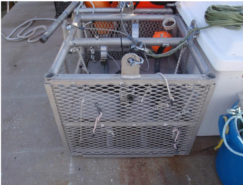
Figure 6. Stereo camera pod. Two cameras are placed inside, each facing 180^\circ to the other. There are also GoPro cameras positioned on the adjacent sides to record surrounding habitat; the four cameras together provide a 360^\circ view.
