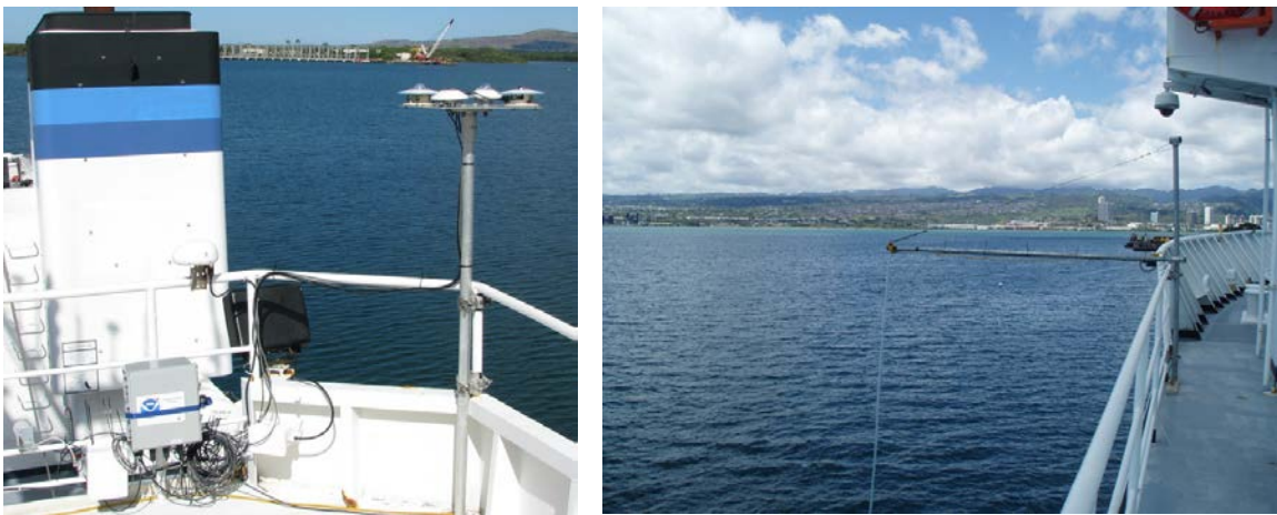
Figure A-2. ESRL/PSD radiometers (left) mounted on deck above the pilot house and the “sea snake” (right) mounted port side of first deck on Hi'ialakai .
