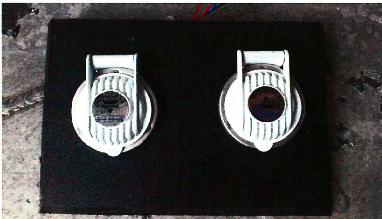
Figure 11. The foot switch for the pinch puller with buttons for UP (right side) and DOWN (left side).
