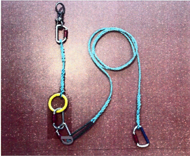
Figure 6. Bottom line set-up with blue clip (attaches to weight), green loop (for green line), and yellow ring (for yellow line to clip onto). The top hardware (with weak link) attaches to the bottom of the MOUSS harness (underneath the MOUSS) during deployment.
