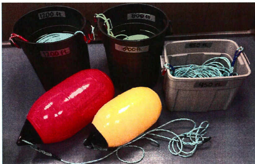
Figure 5. Surface line at lengths of 450 ft, 800 ft, and 1200 ft, stored in and deployed from line bins. One large red surface buoy and one smaller yellow surface buoy are attached to the surface line during deployment.
