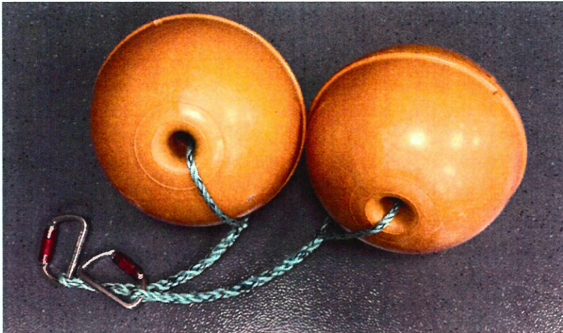
Figure 3. Sub-surface buoys, clipped onto the MOUSS harness during deployment.
