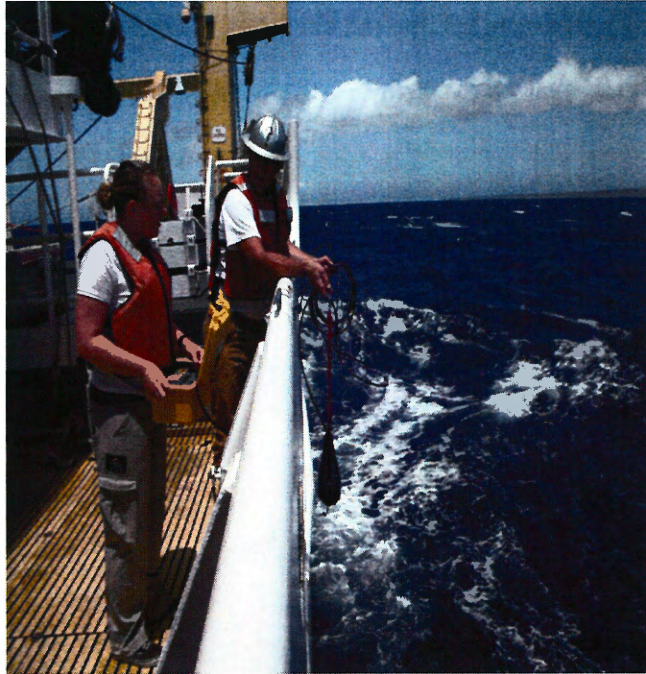
Dunking transducer and deck box for signaling the Acoustic Release.
