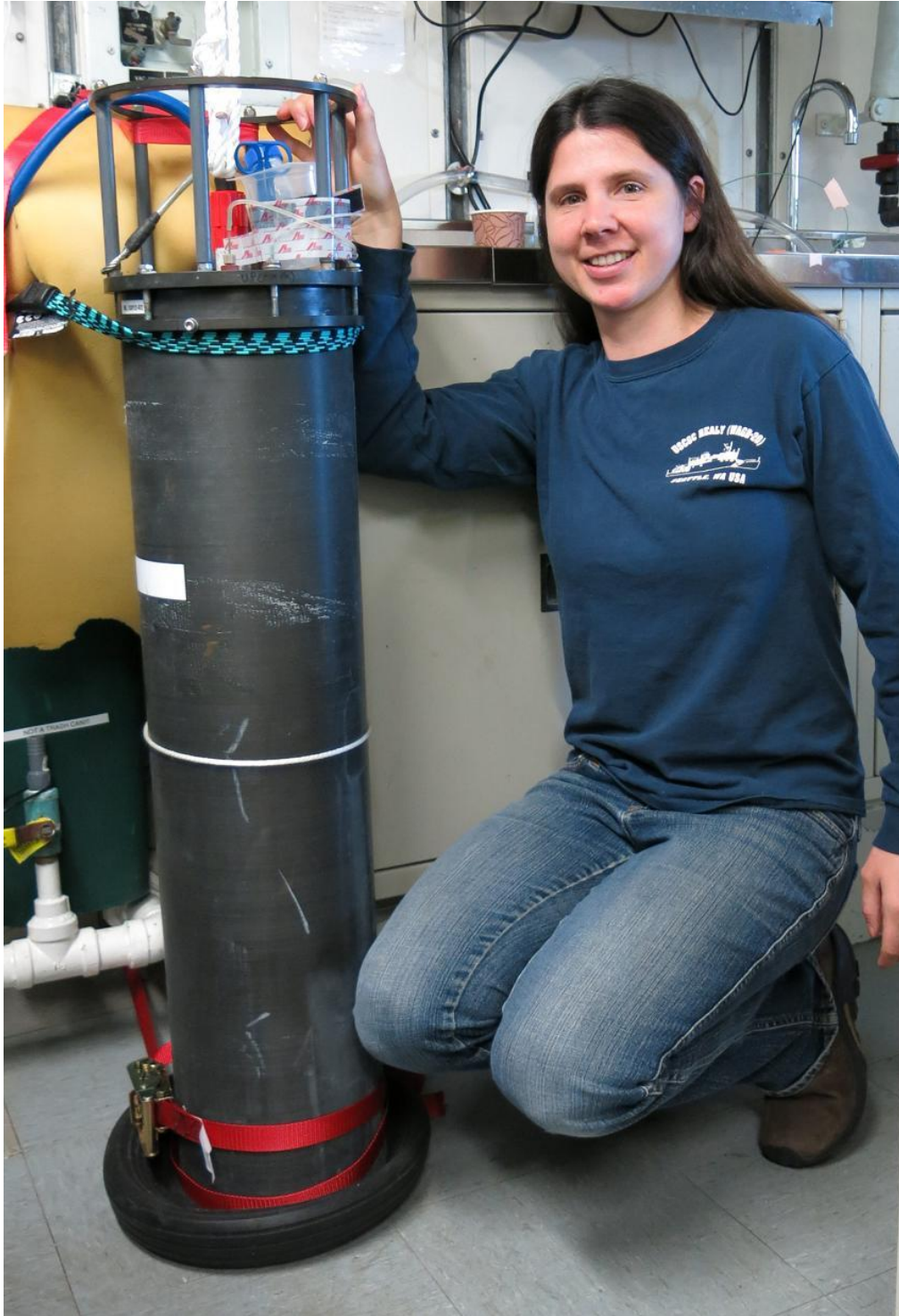
Figure 4. The cylindrical Imaging FlowCytobot unit.
