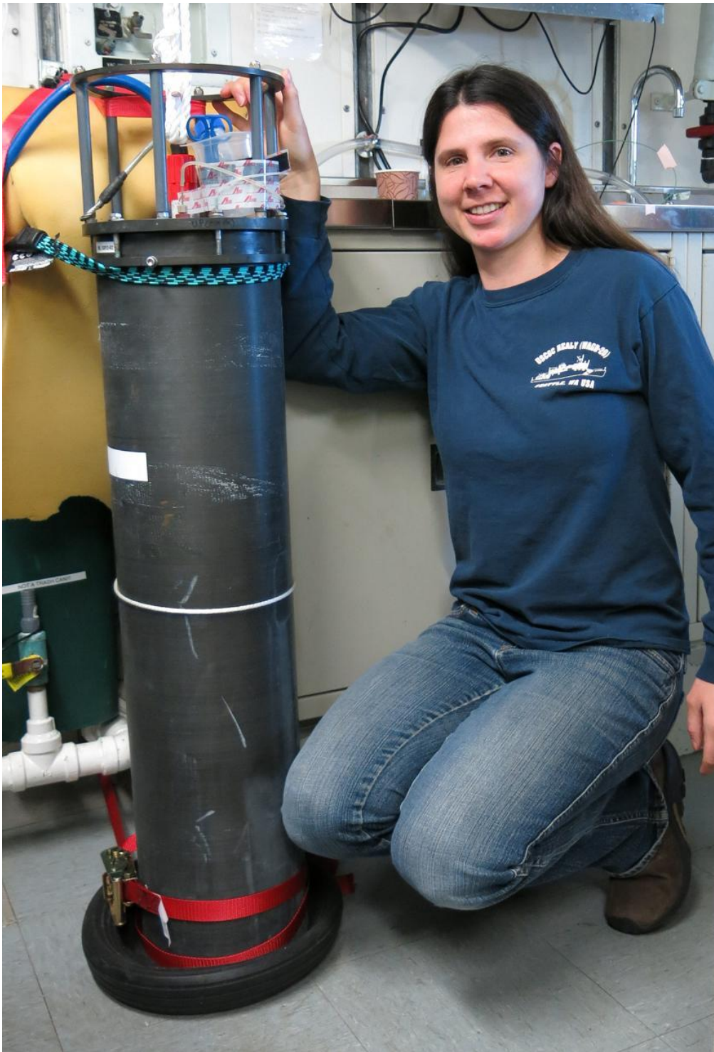
Figure 4. The cylindrical Imaging FlowCytobot unit.
