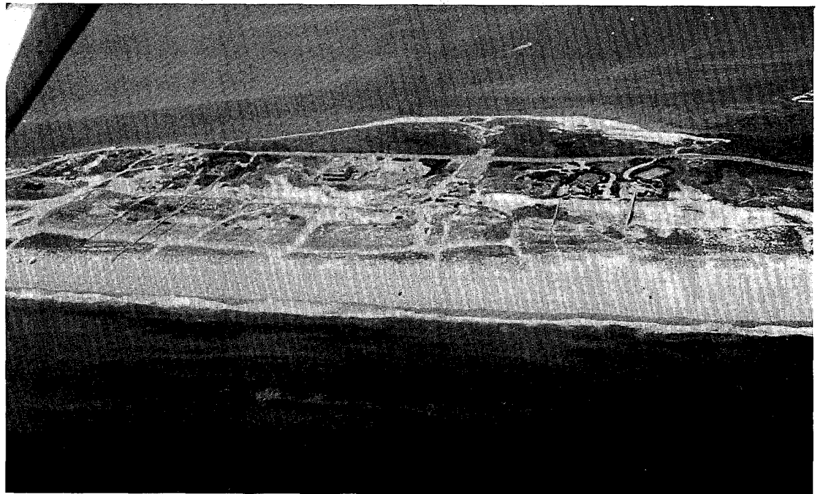
FIGURE 3-27 - Southampton Barrier Spit, July 1989. Note extensive beach width immediately updrift of Shinnecock Inlet and newly constructed mansions located in CBRA designated area
