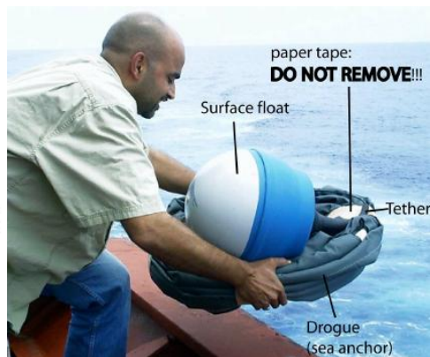
Fig. 2: Drifter schematic in water, left, and at deployment, right. (Lumpkin, R. and M. Pazos, 2006: Measuring surface currents with Surface Velocity Program drifters: the instrument, its data, and some recent results. Chapter two of Lagrangian Analysis and Prediction of Coastal and Ocean Dynamics (LAPCOD) ed. A. Griffa, A. D. Kirwan, A. J. Mariano, T. Ozgokmen, and T. Rossby.)
