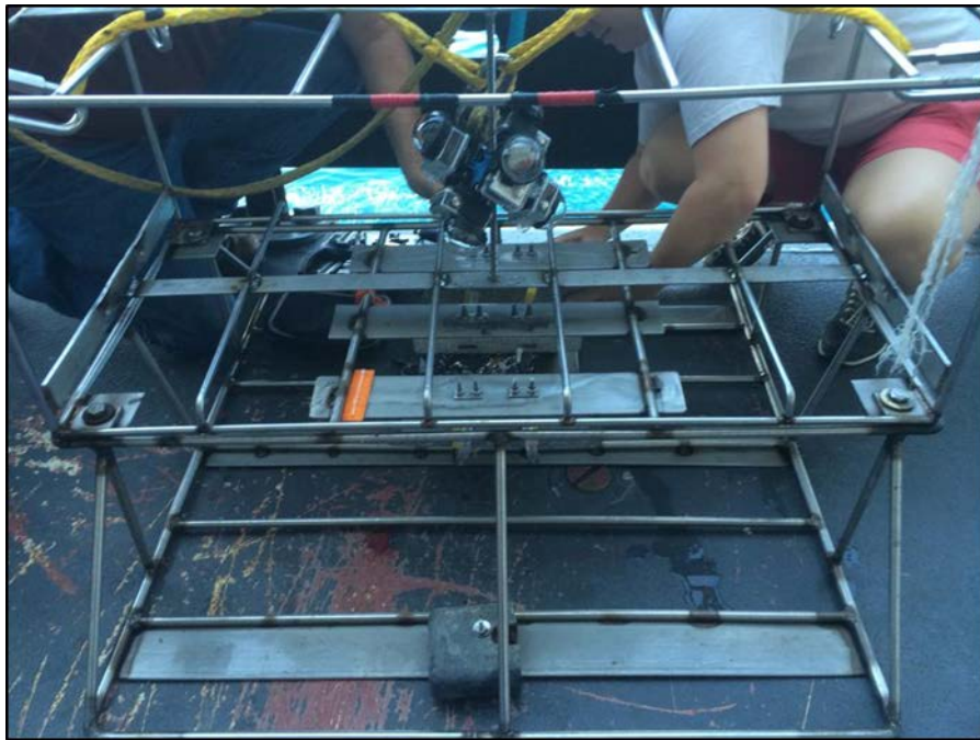
Figure 3. Picture of the SUMO video camera array showing the camera mount (top) and the cage system in which the system is deployed (bottom).
