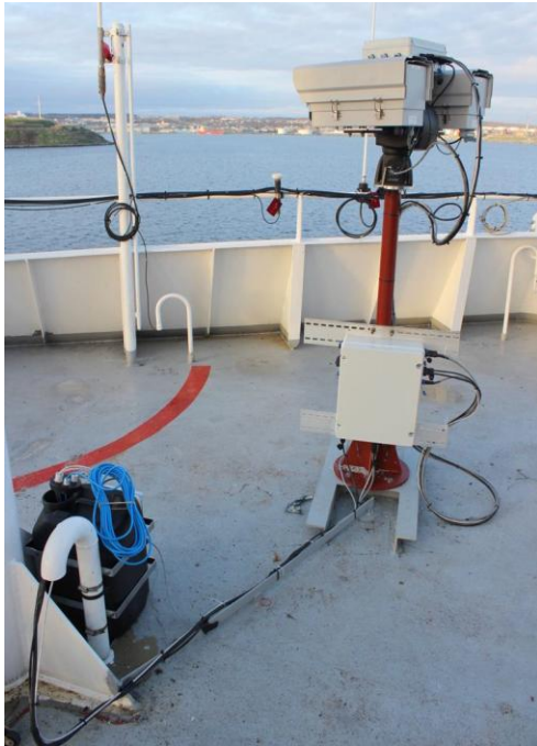
Figure 3. Infra-red camera system that will be utilized during survey to scan for detections of cetaceans.
