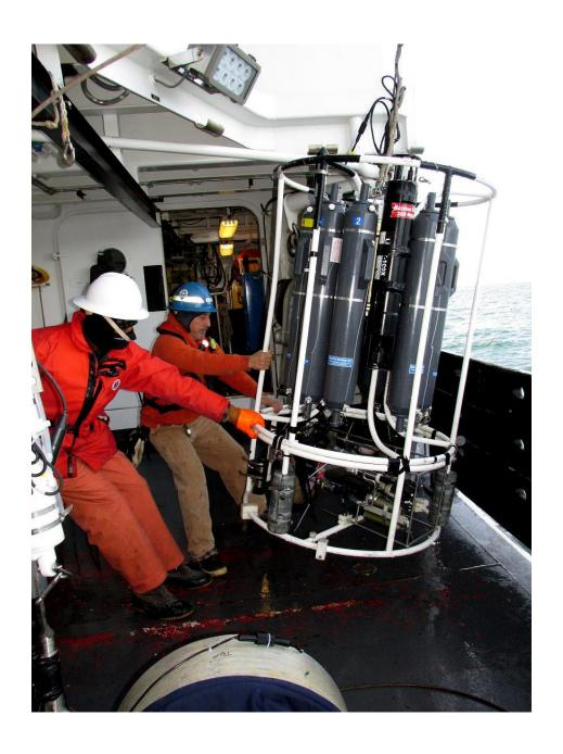
Figure 3. A Niskin bottle rosette sampler equipped with 10 liter Niskin bottles.
