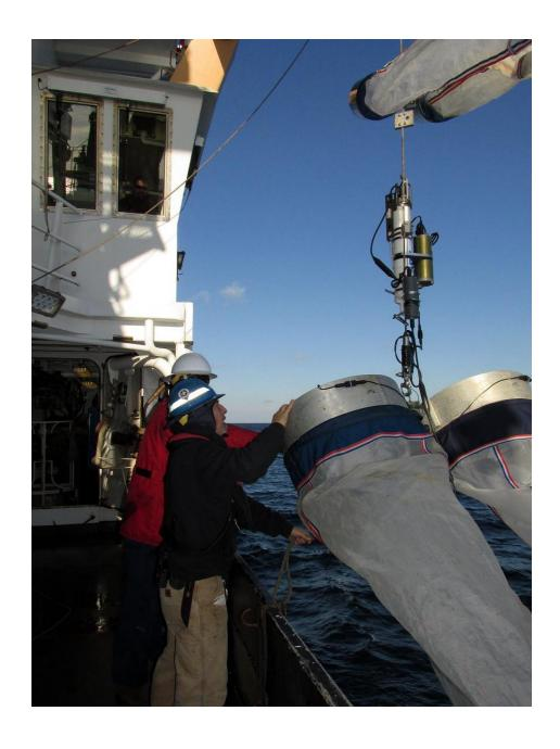
Figure 2. Plankton net sampling array, showing 61 and 20 cm bongo frames, and CTD unit.
