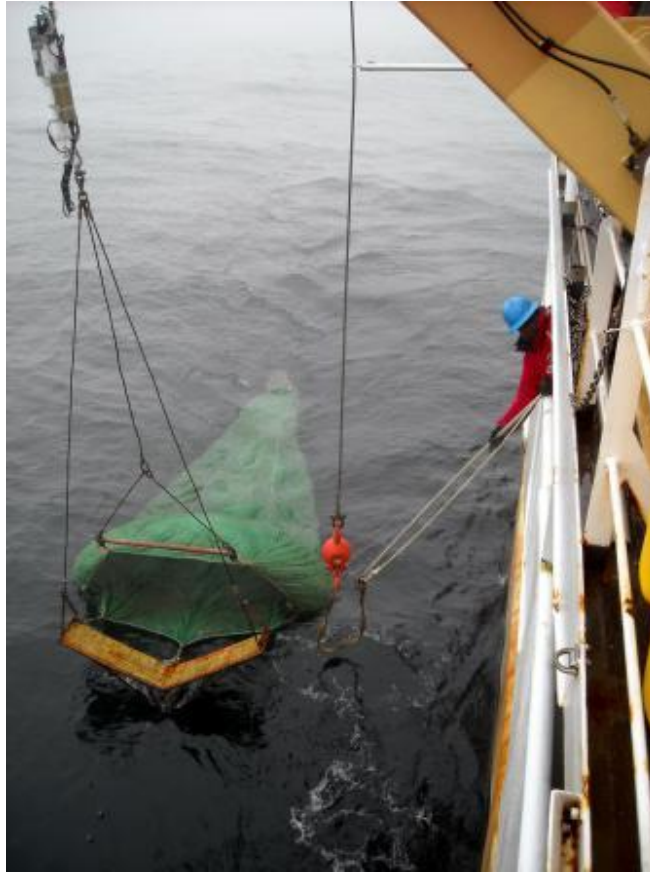
Figure 2. Six foot wide Isaacs Kidd Midwater Trawl.
