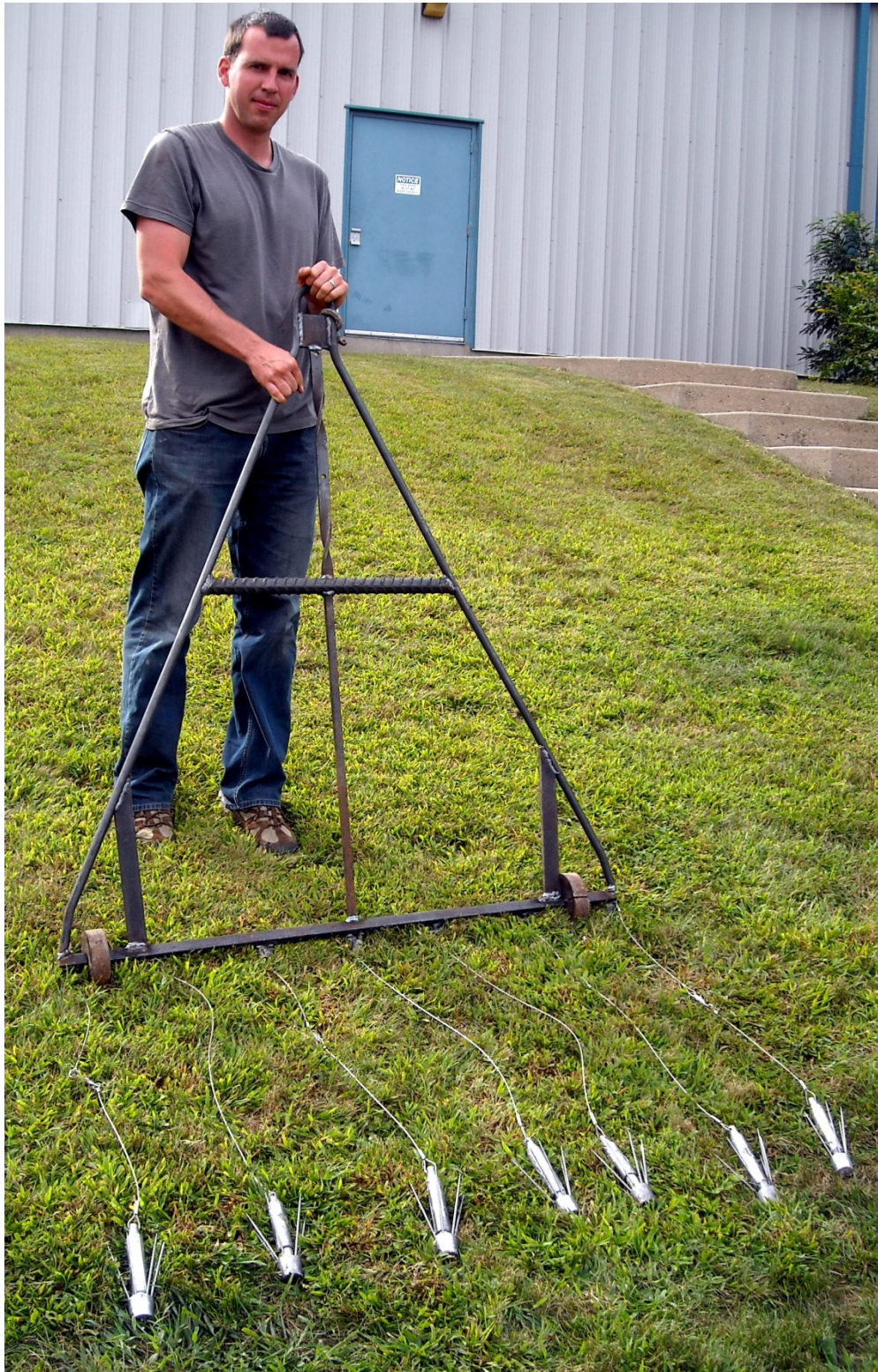
Figure 4. Dave Richardson-modified Karatsuri Sand Lance Collection Rake
