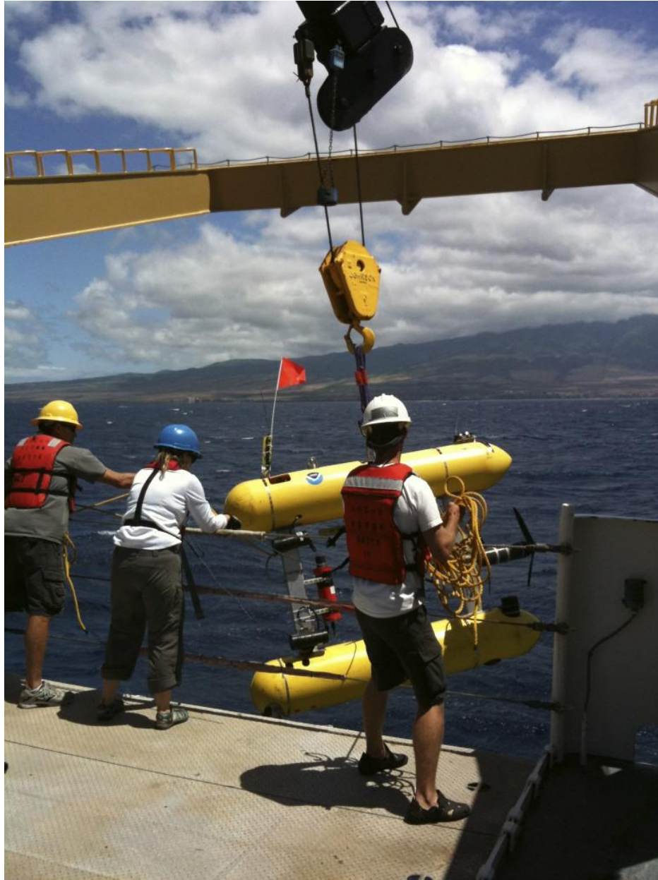
Fig. 4. Deploying the AUV from the fantail
