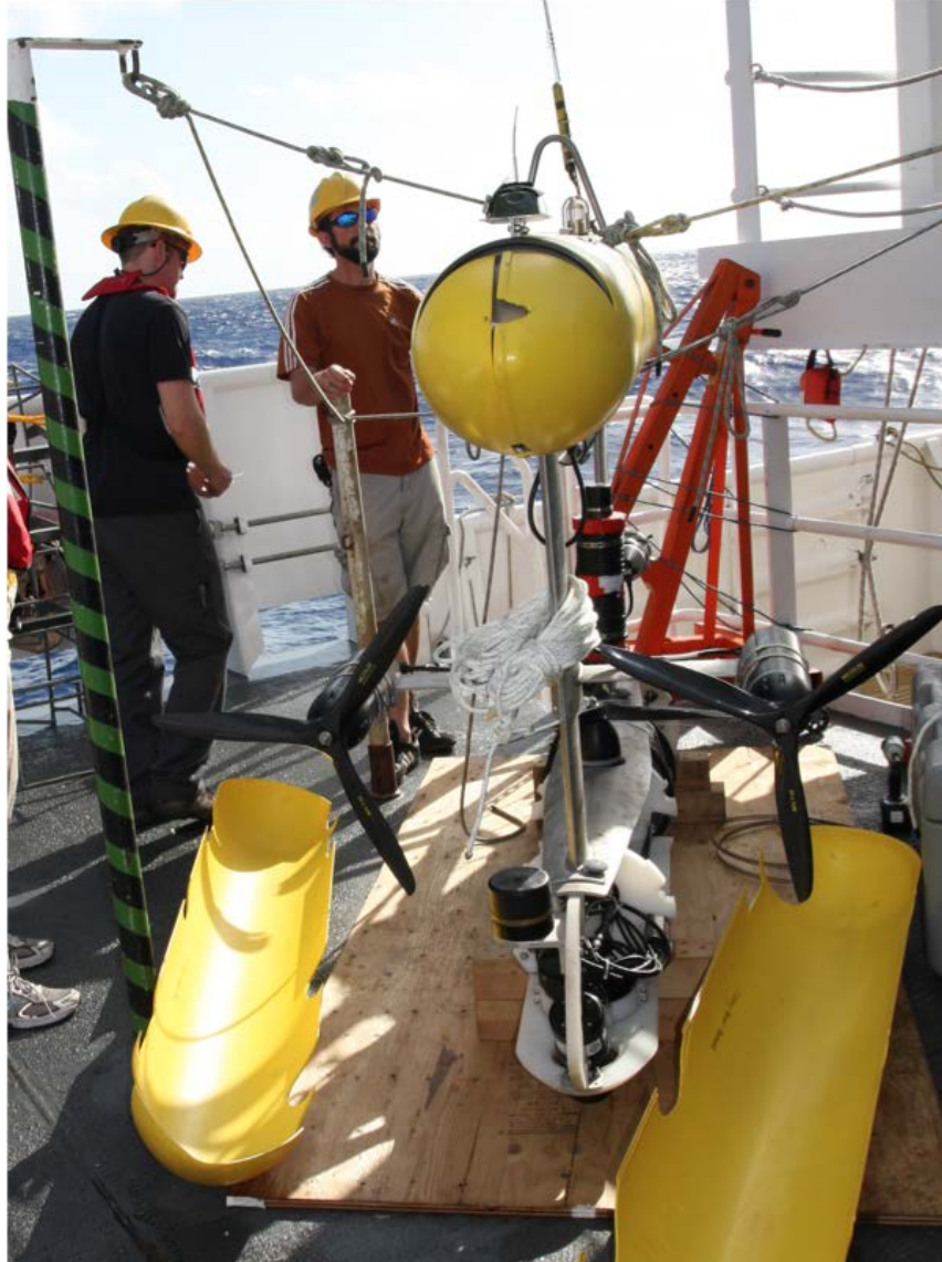
Fig. 2. AUV on deck tied to stanchions with lower skins off
