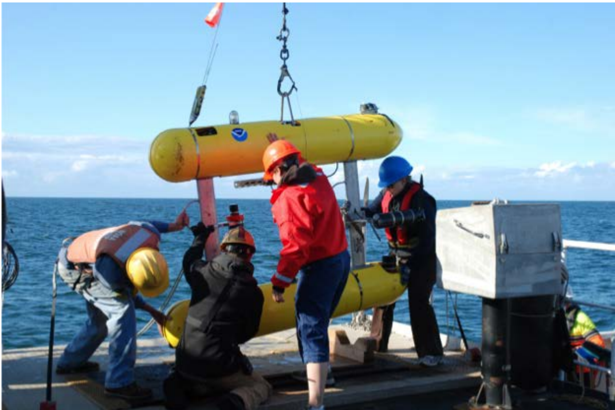
Fig. 1. AUV Lucille being placed in cradle on deck.
