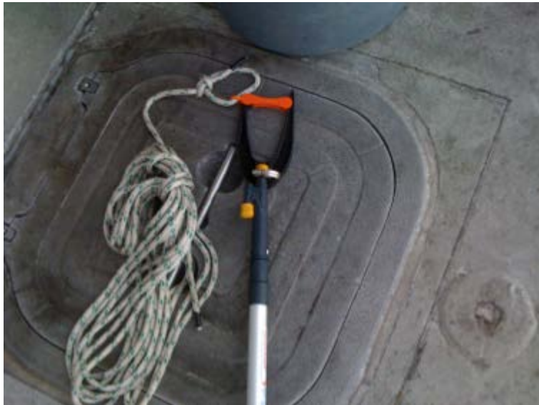
Fig. 6. Happy Hooker attached to pole
