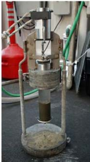
Figure 4. NIOZ moncore which will be suspended under the CTD carousel by a 10 m line. The mono-core weighs about 40 kg (= 88 lbs).
