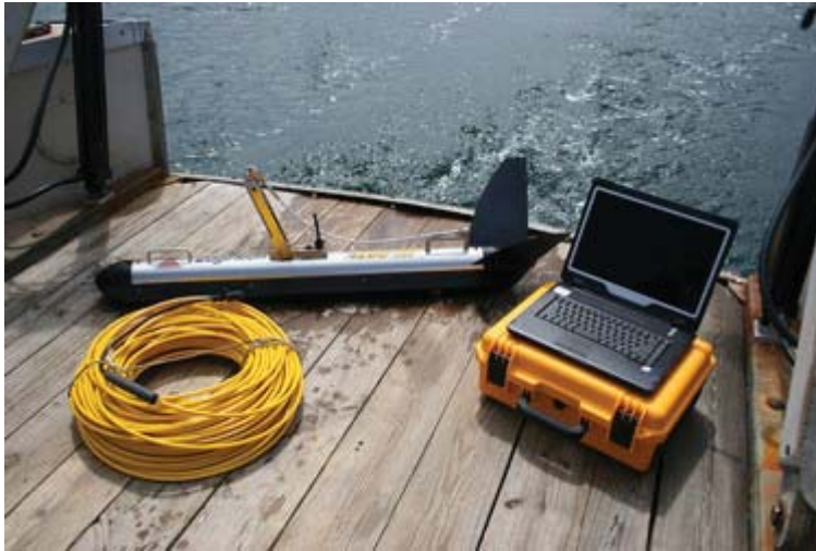
Image of Edgetech 4200 Sidescan Sonar towfish
