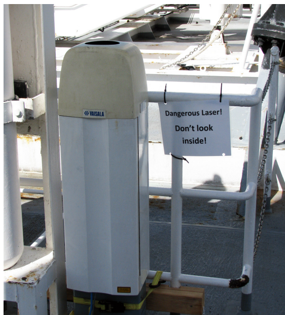
Figure A-3. ESRL/PSD ceilometer mounted on the HA deck.
