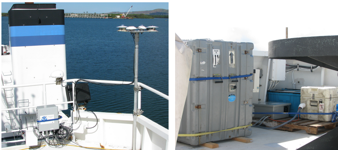
Figure A-2. ESRL/PSD radiometers (left) and electronics packages (right) mounted on deck above the pilot house on the Hi'ialakai .
