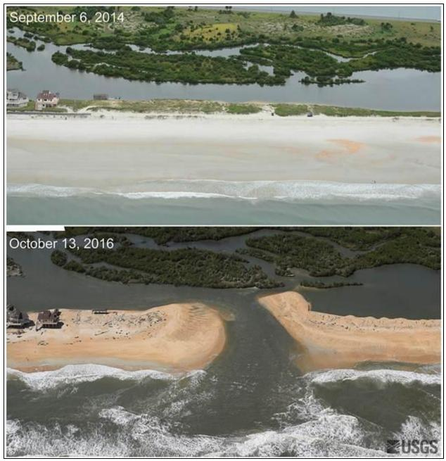
**Figure 11:** Low-altitude oblique photos taken before Hurricane Matthew (September 6, 2014) and after (October 13, 2016) showing where the storm cut a new inlet between the Atlantic Ocean and the Matanzas River, stripping away 12-foot dune and carrying sand into the estuary. *Source: USGS*
