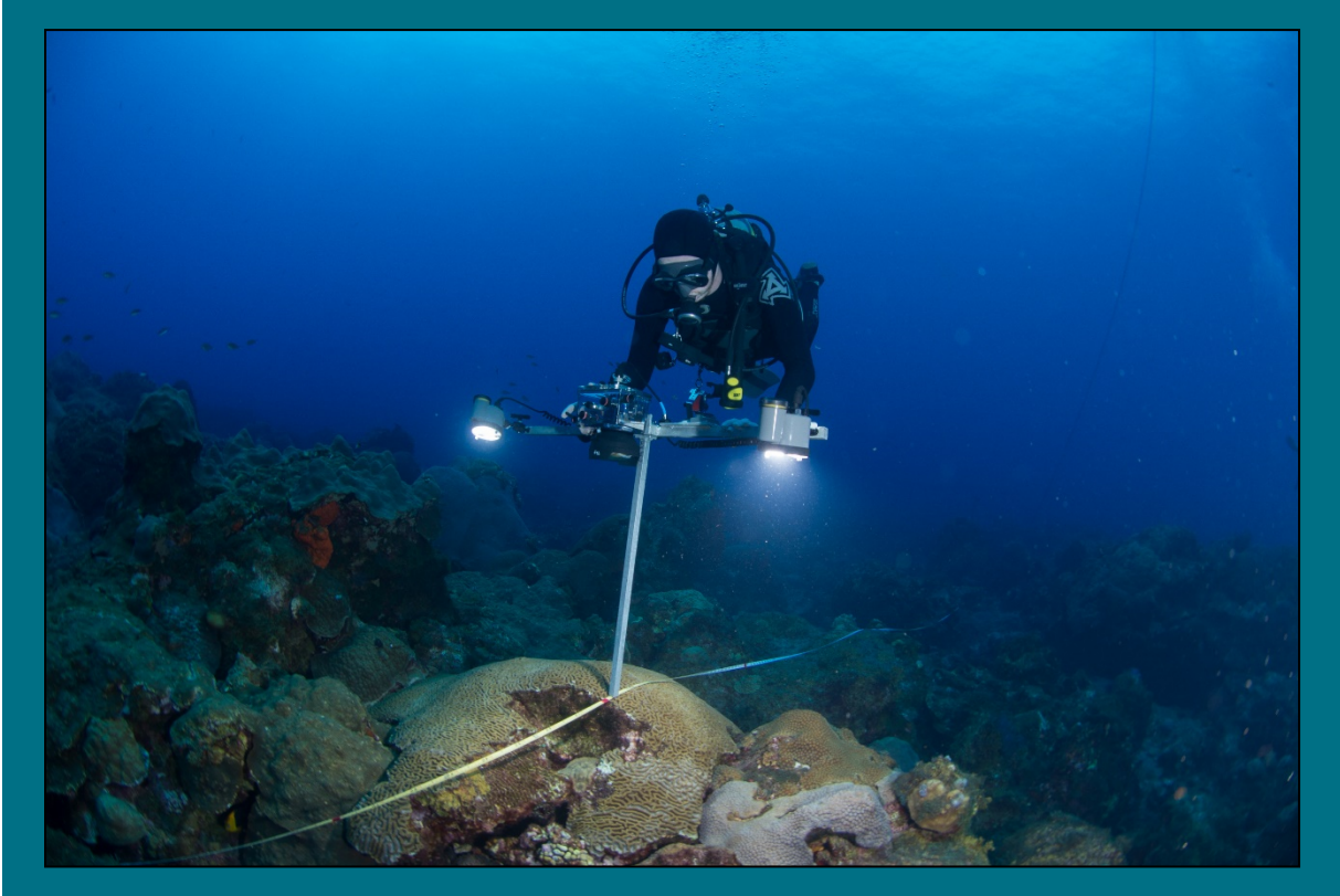
NOAA diver, Ryan Eckert, with camera and strobes mounted on aluminum t-frame taking random transect photographs within the East Flower Garden Bank study site. (Photo: G.P. Schmahl, NOAA/FGBNMS)
