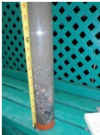
Fig. 2 Photograph of a core from Benner Bay illustrating the change in texture from shell hash to fine-grained sediment over time
