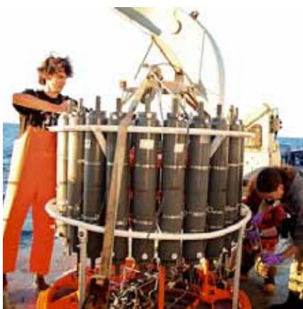
Ben Grupe begins to prepare the CTD bottles for deployment, an instance when being tall comes in handy. Normally, scientists have to climb onto the white frame to cock the bottle caps. As the CTD is lowered into the ocean, a computer is used to watch the data and order bottles to snap shut, collecting water samples from different depths. Image courtesy of NOAA's INSPIRE: Chile Margin 2010.
