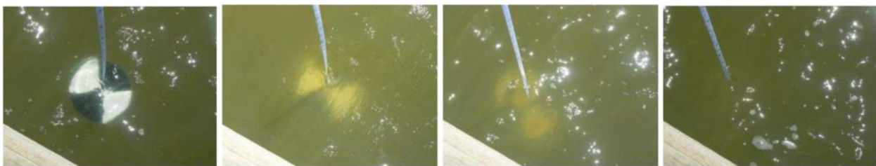
Figure 16. A Secchi Disk Measure of Water Clarity is the Depth at Which a Disk is Visible when Submerged in Water.
