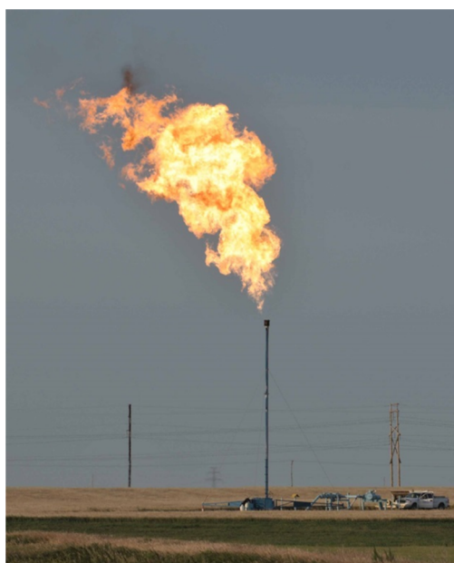
Figure 1. Large quantities of radiant energy are produced by gas flares.
