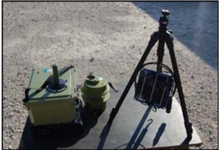
The Weather Pod meteorological sensor system for remote locations. Photo courtesy U.S. Air Force Weather.
