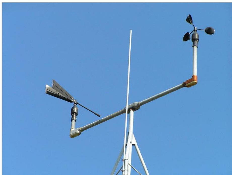
Figure 2-3. Close-up of a cup anemometer (photo courtesy of NOAA/NWS).
