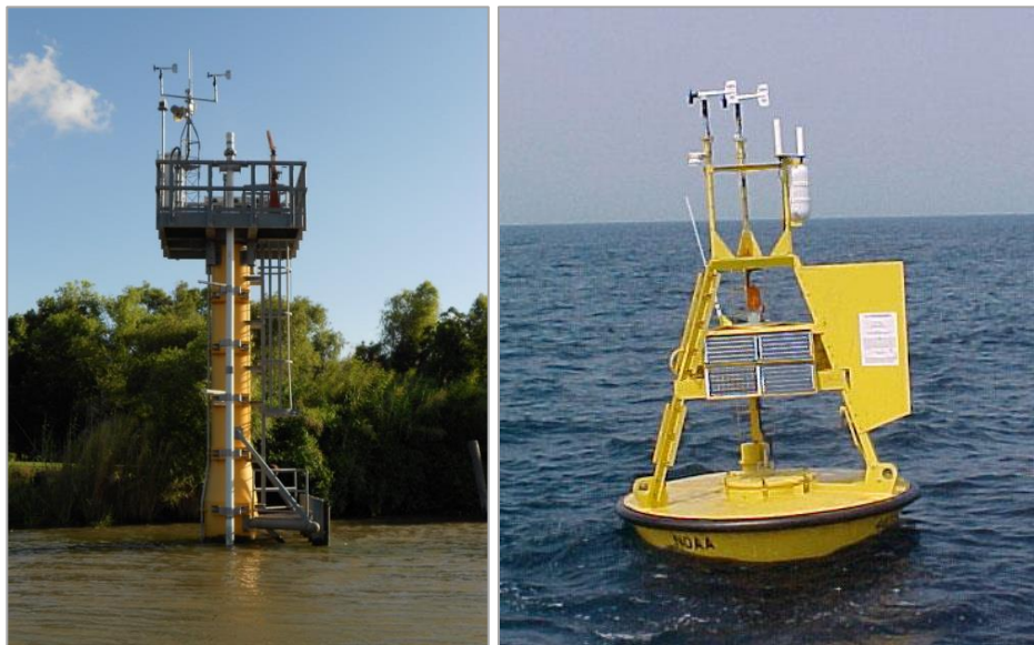
Figure 2-2. Example of a vane anemometer atop a fixed platform (L) (photo courtesy of NOAA/CO-OPS) and on a moored buoy (R) (photo courtesy of NOAA/NDBC).
