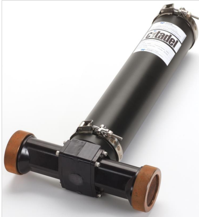
Figure 2-5. The Teledyne RD Instruments CITADEL CTD-NH is an example of an inductive sensor with a constrained field (photo courtesy of Paul Devine/Teledyne RD Instruments).
