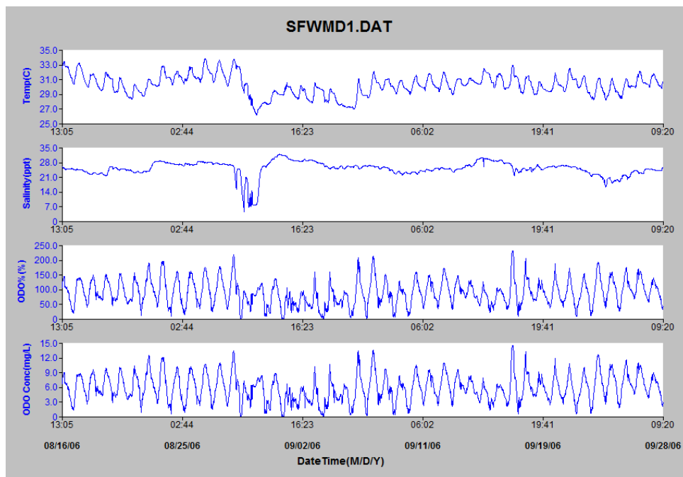
Figure 2-1. Panels 1-4 show temperature, salinity, DO percent, and DO concentration, respectively. The series tracks the passage of a hurricane and the effect it has on the time series before, during, and after the storm front passes (courtesy of Mike Lizotte, YSI).
