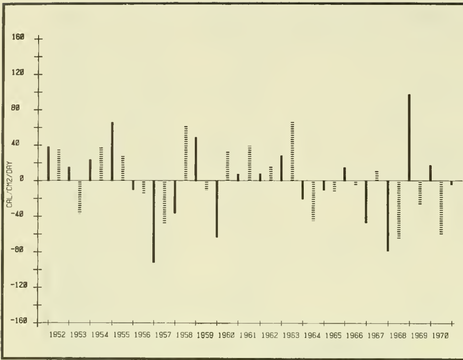
Figure 7.—Seasonal anomalies of net heat exchange at Ocean Weather Station V (OWS-V), October 1951-March 1971, for 6-mo cooling (solid bar) and 6-mo warming (dashed bar) portions of the annual cycle. Anomalies are relative to the 1952-70 mean values. Values prior to April 1955 were adjusted for the change in latitude of OWS-V.
