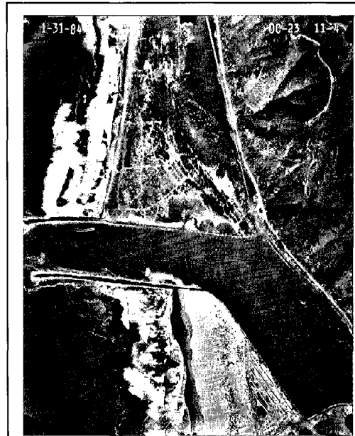
Figure 23. Effects of Man-Made Structure on Longshore Current
