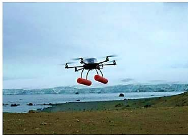
Figure 82. One type of unmanned aerial system that has been used in the field for marine mammal research: the APH-22 Hexa-copter.
