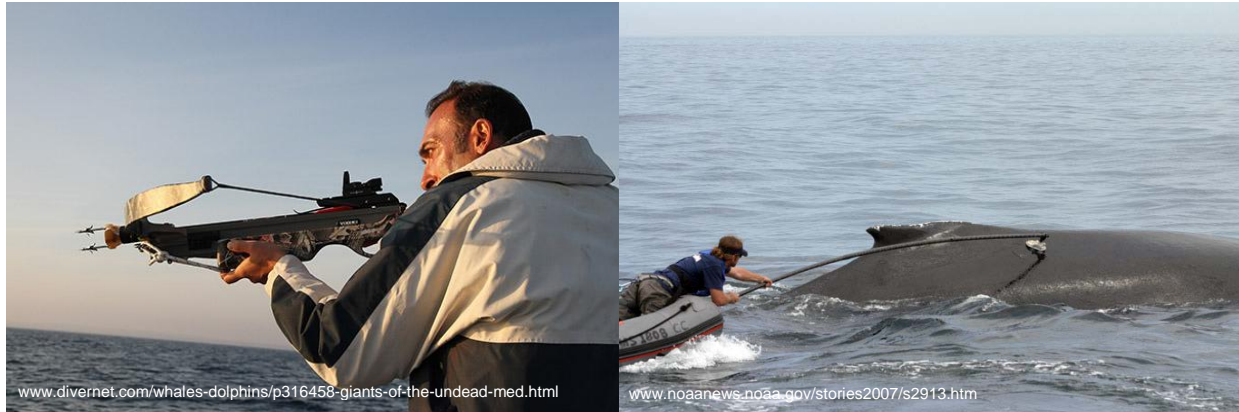
Figure 3: Example of crossbow equipped with Low Impact Minimally Percutaneous External-electronics Transmitter tag (left), and example of suction-cup tag deployment with hand-held pole (right).
