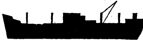
General Cargo Liner 1/ "Salty" Length = 500' Beam = 75' Draft = 24' Cargo tonnage = 9,000
