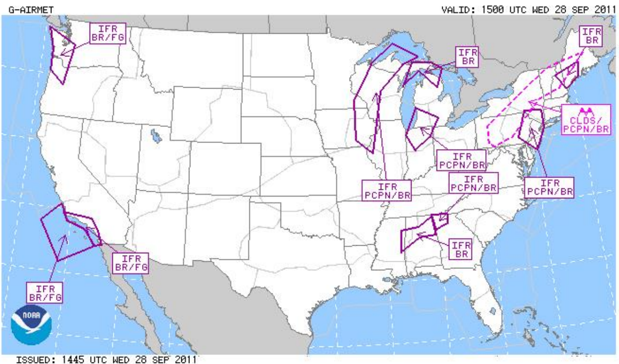
Fig. 3.2. A graphical AIRMET for Instrument Flight Rule (IFR) conditions, valid at 1500 GMT, 28 Sep 2011. The three polygons in the Upper Midwest and covering parts of the Great Lakes were also discussed as a text file above. The abbreviations BR, FG, PCPN, and CLDS mean mist, fog, precipitation, and clouds, respectively. The dashed pink outline over parts of the
