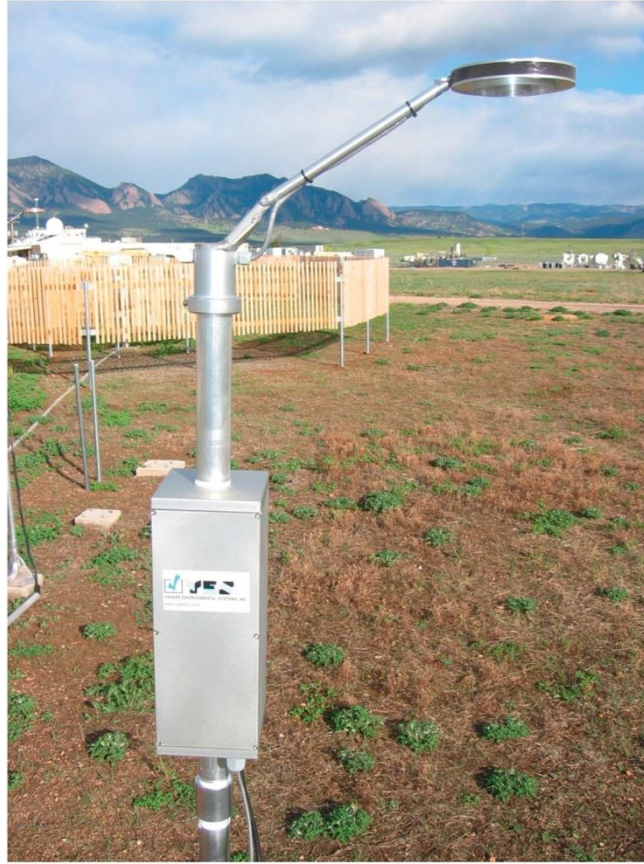
Fig. 3.36. A commercial version of the hotplate precipitation gauge, manufactured by Yankee Environmental Systems. From Rasmussen et al. (2011). Reprinted with permission of the American Meteorological Society.
