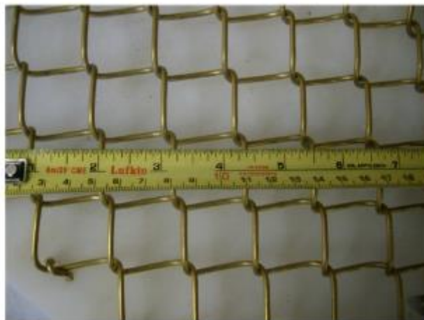
Figure 7. Copperalloy mesh for the Sides and Bottom of the Velella Delta Array. (Source: Kampachi Farms, 2014)
